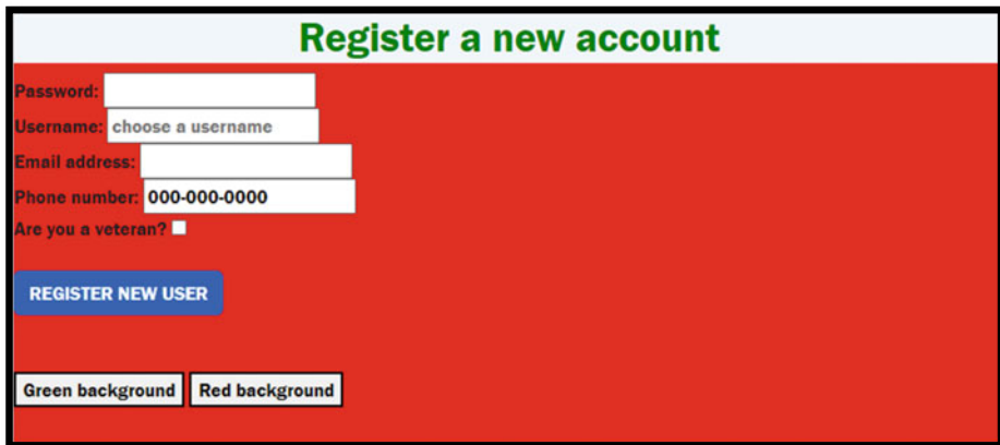
Fig. 4.23 The webpage has a red background after the user clicks on the “Red background” button
