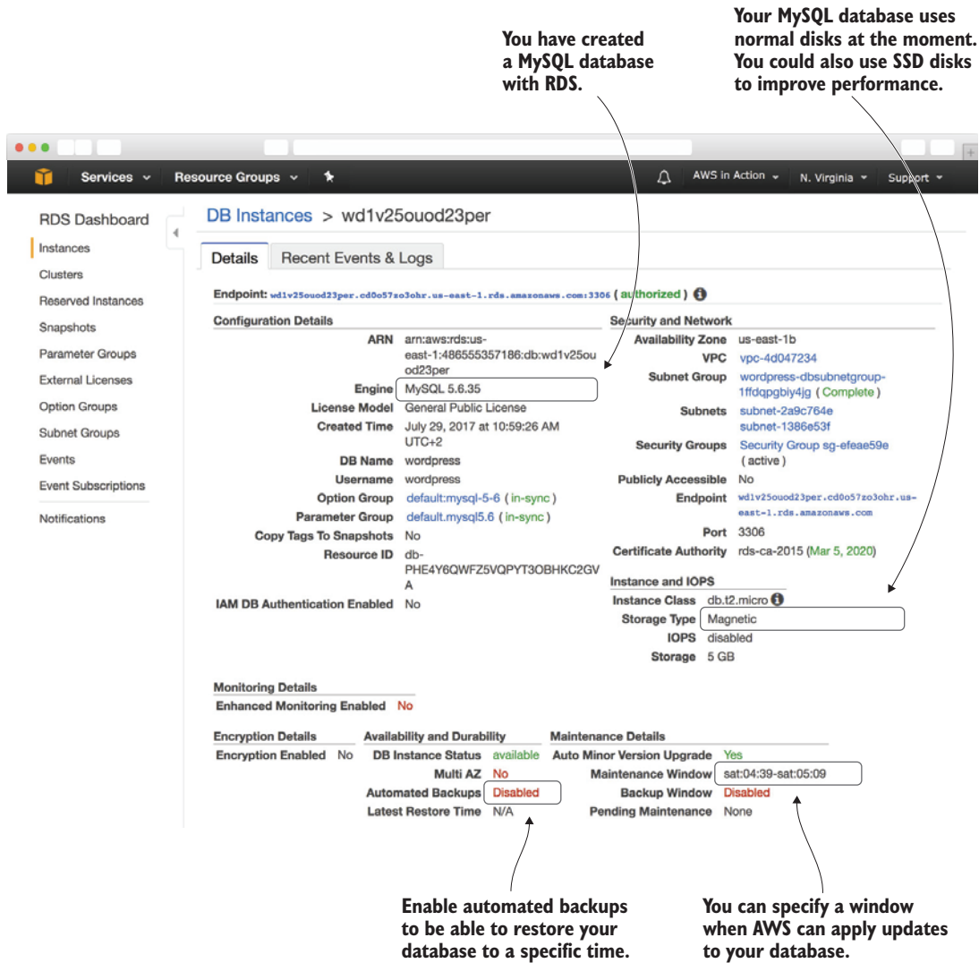
Figure 2.16 Details of the MySQL database storing data for the blogging infrastructure
