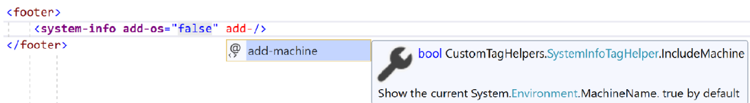
Figure 20.2 In Visual Studio, Tag Helpers are shown in a purple font, and you get IntelliSense for properties decorated with [HtmlAttributeName] .
