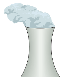
The shape of a cooling tower is a hyperbola.
