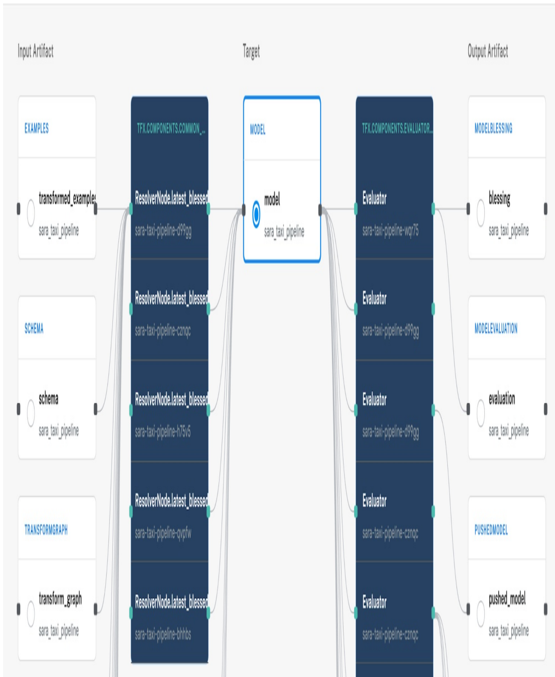
Figure 6-11. The Lineage Explorer section of the AI Platform Pipelines dashboard for a TFX pipeline.
